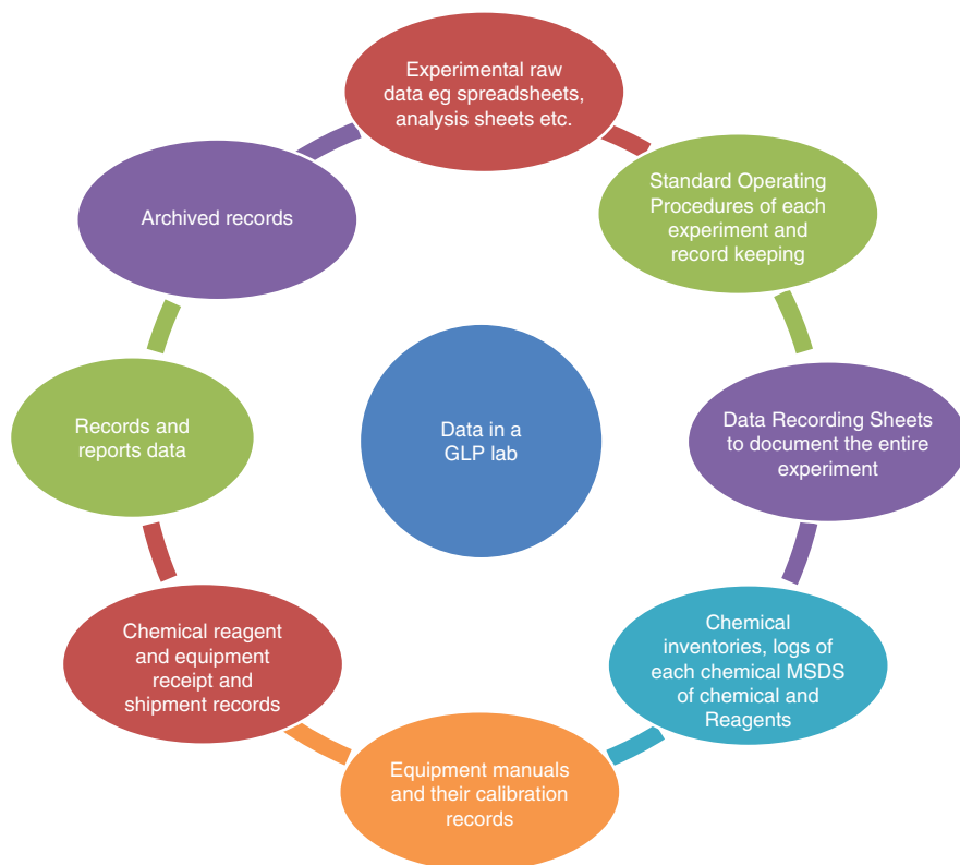
Fig. 13.1 Type of data generated in a GLP compliant lab. Maintenance of data in this format allows easier and convenient workflow in a laboratory. GLP documentation practices also generate enough evidence of the data to ensure its integrity and reliability. GLP, good lab practices
