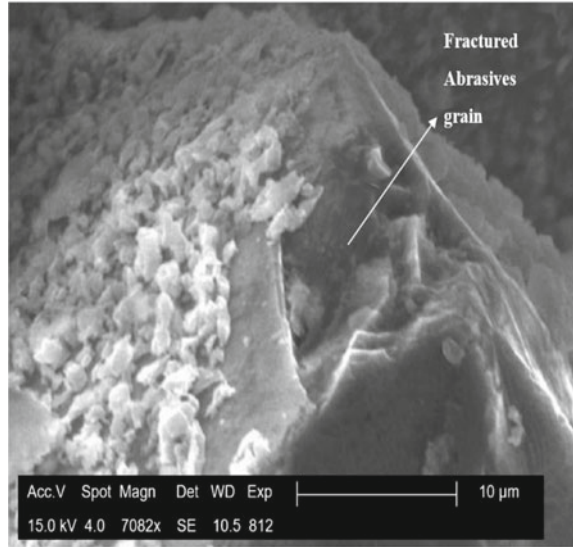
Fig. 10 Tear-out of diamond grit from the tool
