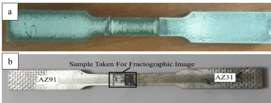
Fig. 4 Tensile test sample, a initial (before finishing); b after test
