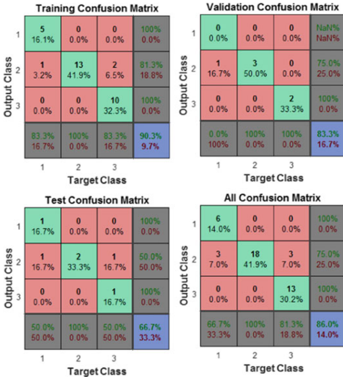
Fig. 7 Confusion plot obtained through the NNs during the grinding of mild steel workpiece
