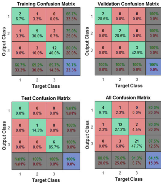
Fig. 6 Confusion plot obtained through the NNs during the grinding of aluminium workpiece
