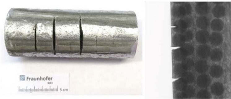
Fig. 5 X-ray transmission image for better visualization and understanding of cutting effect [15]
