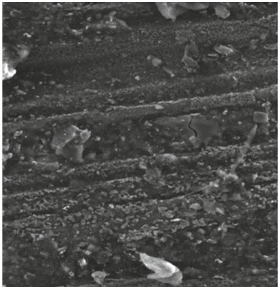
Fig. 5 SEM image (100X) of 98% Al + 2% B_4C
