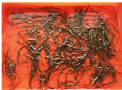
a) Fiber soaked in NaOH solution
