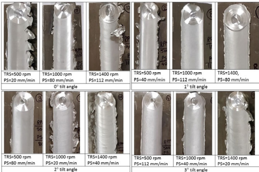
Fig. 5 Formation of flashes in the FSPed sample at different TA
