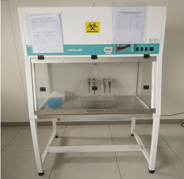
Fig. 13.1 Class II A2 cabinet. (Source: This work)
