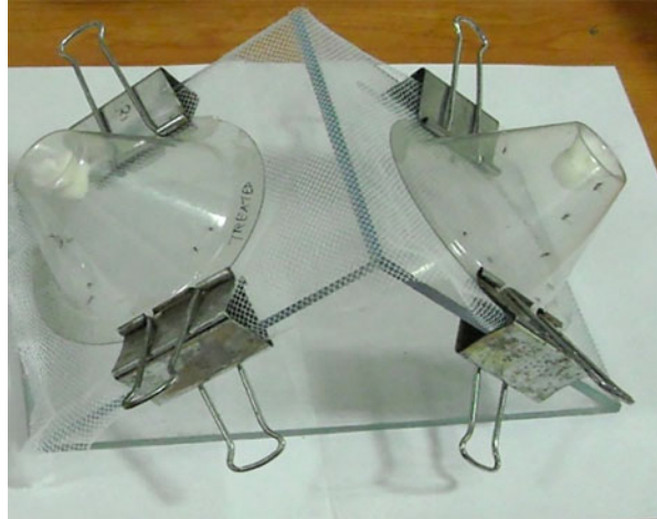
Fig. 16.2 WHO cone bioassay for mosquitoes using LLIN. (Source: This work)
