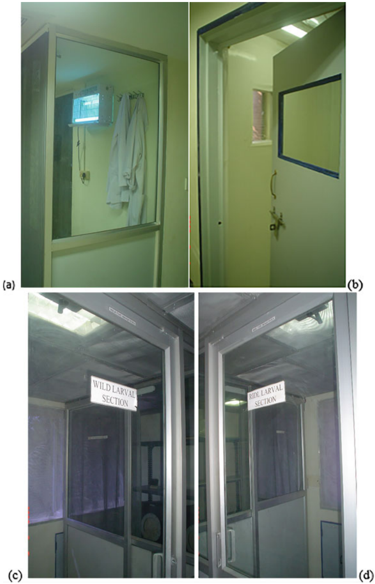
Fig. 7.1 Arthropod Containment Laboratory essentials for biological experiments on RIDL and wild Aedes aegypti populations, (a) mating chamber, (b) anteroom, (c) wild larval section, (d) RIDL larval section, (e) double curtain, (f) air curtain and (g) AC with net covering. (Source: This work)
