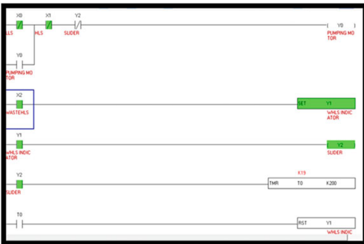
Fig. 7 PLC output when WLS-ON, servo motor-ON
