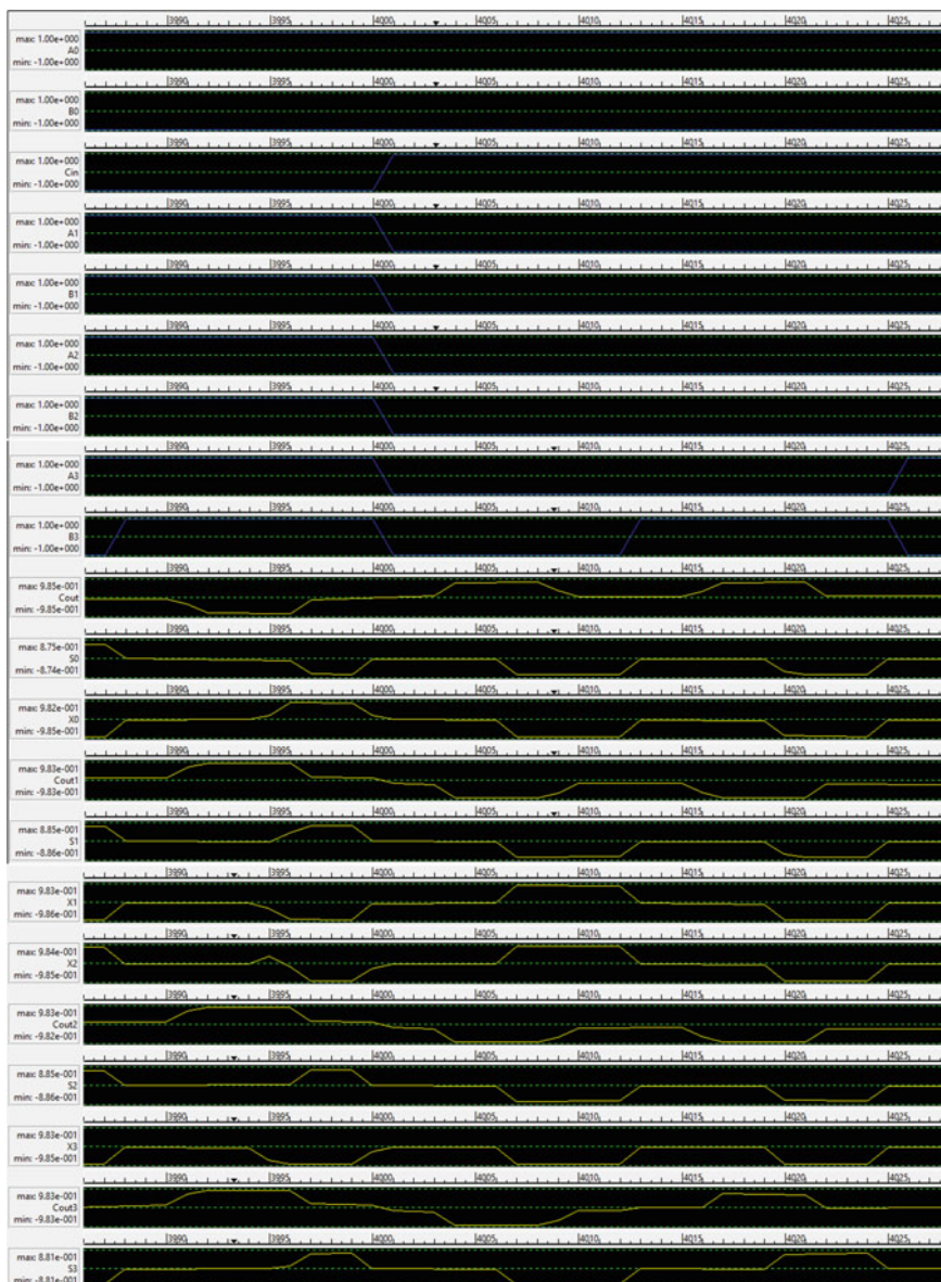
Fig. 9 Output of four-bit reversible multilayer "RCA" design with "XOR" operation
