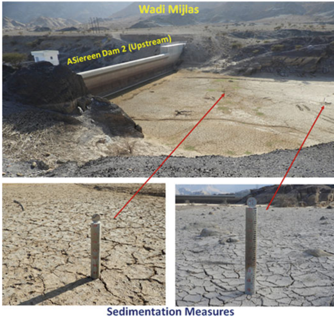
Fig. 15.7 Sedimentation measures at the reservoir of Asserin Up Dam at the upstream of Wadi Mijlas (photographs taken by the Kyoto University team: field survey from Nov. 29 to Dec. 2, 2017). Reprinted from Saber et al. (2018), Copyright 2018
