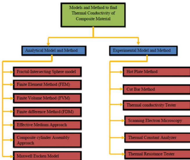
Fig. 3.1 Experimental and analytical method and model for finding thermal conductivity of composite material
