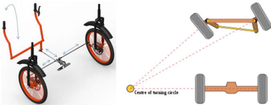
Fig. 2.7 Steering system overall geometry [11, 12]
