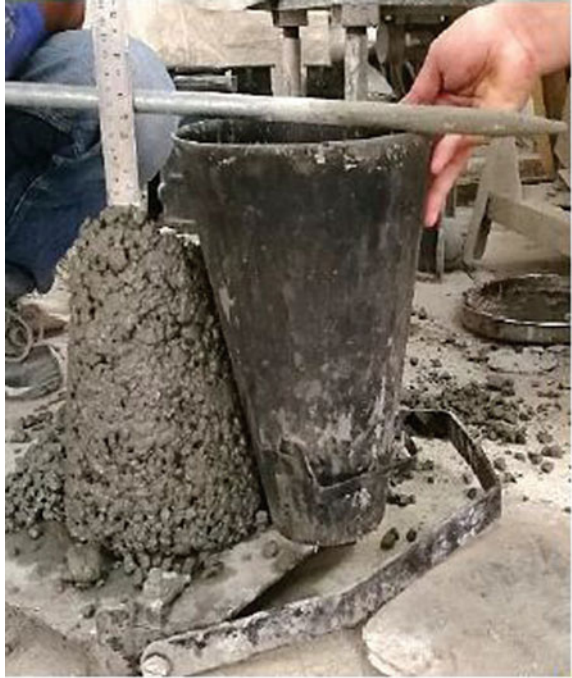
Fig. 3 Experimental setup for slump test
