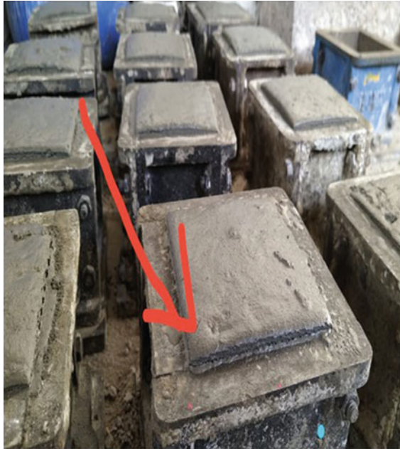
Fig. 1 Cube specimens with aluminium dross (noticeable swelling at 10% can be observed)
