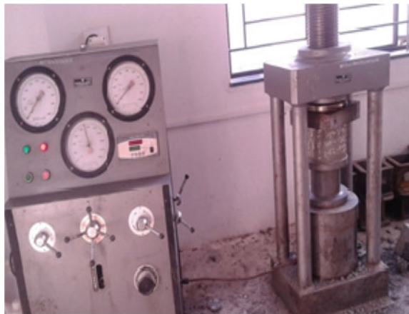
Fig. 3 Compressive strength test setup
