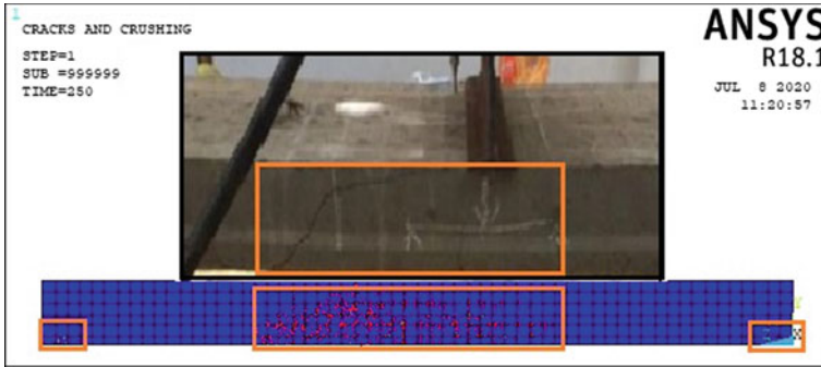
Fig. 15 Crack patterns observed under LL
