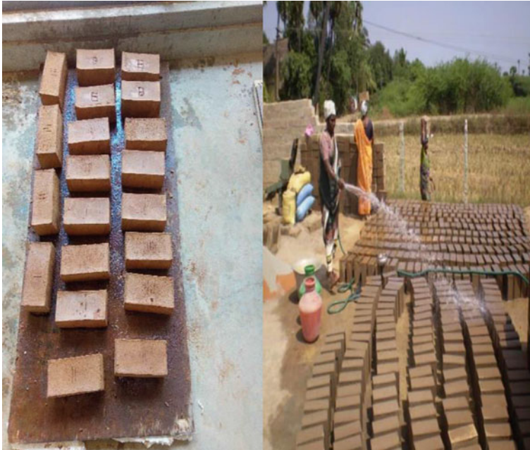
Fig. 2 Demoulded adobe bricks (right) and curing of adobe bricks (right)
