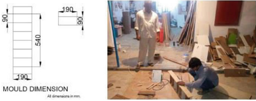
Fig. 1 Details of mould (left) and mould fabrication process (right)
