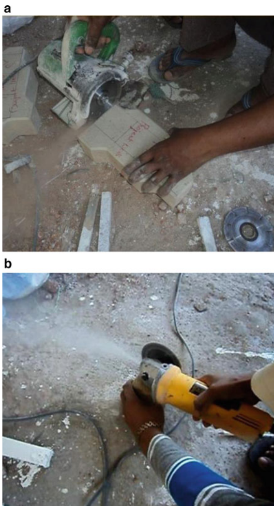
Fig. 9 a Preparation of ICPB specimen for Abrasion Test. b Preparation of ICPB specimen for Abrasion Test
