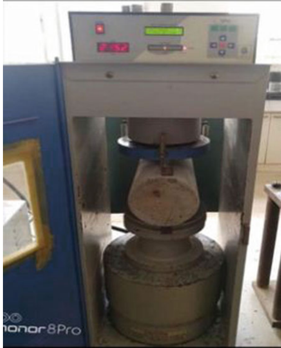
Fig. 5 Experimental setup of split tensile test
