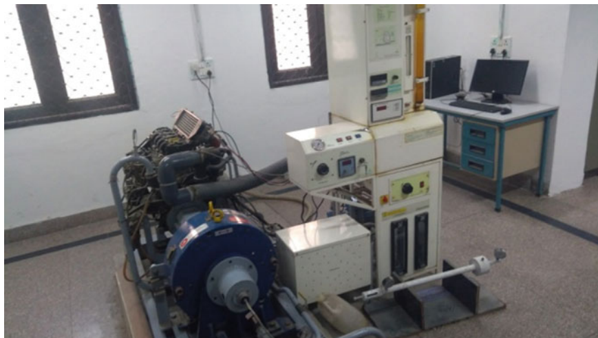
Fig. 1 Four-cylinder, four-stroke TATA turbo engine
