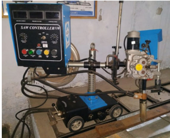
Fig. 1 SAW machine trolley and rail
