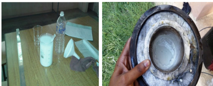
Fig. 4 Slaked \text{Ca}(\text{OH})_2 solution and calcium hydroxide stone deposit after conducting an endurance experiment in the diesel engine
