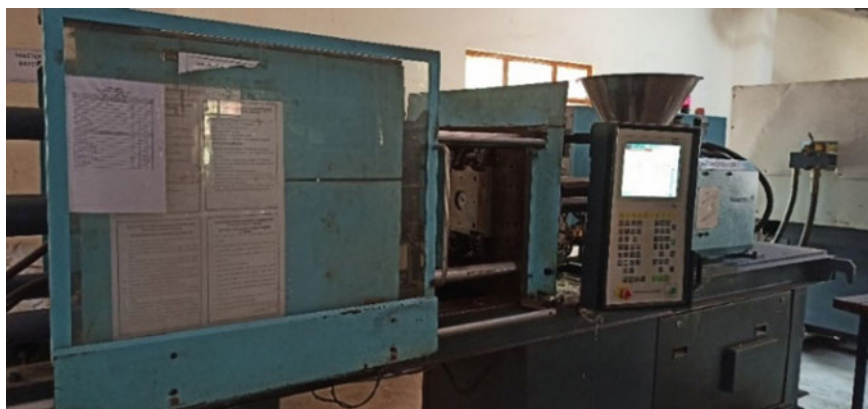
Fig. 3 Injection moulded machine 'De-Tech85 LNC5' at CIPET, Jaipur
