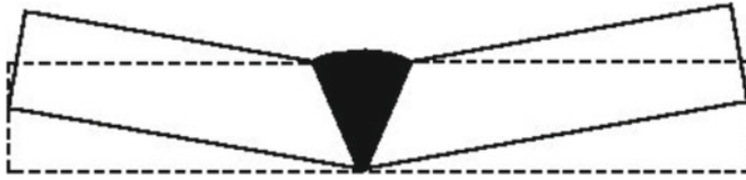
Fig. 1 Transverse section of angular distortion in a plate [6]
