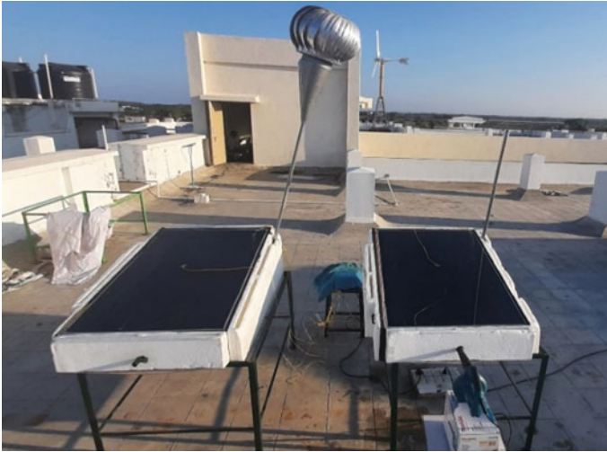
Fig. 1 Single slope forced convection and natural convection solar dryer
