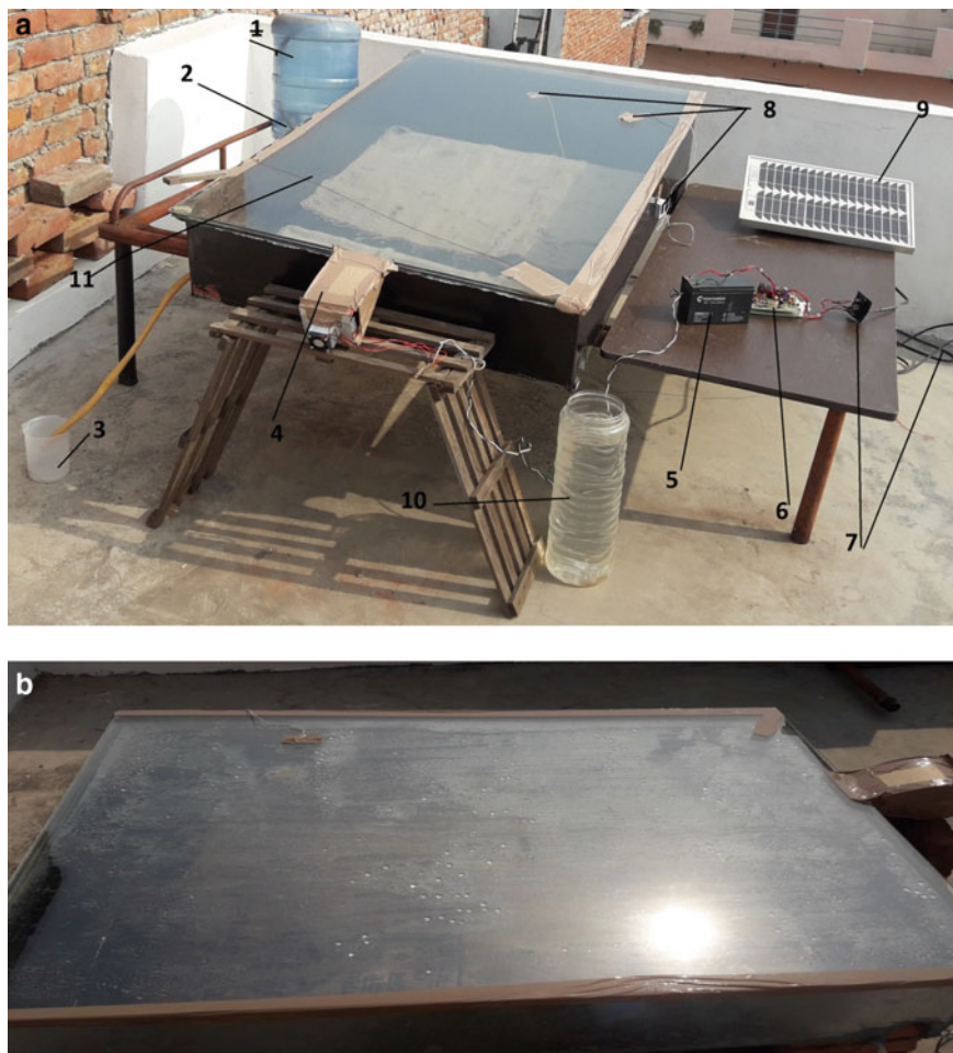
Fig. 3 a Photograph of experimental setup of solar still (1) water input device (2) water circulation (3) condensate water collection (4) cooling fan unit (5) battery (6) inverter (7) AC to DC converter, PVC cable (8) temperature measuring device (9) solar plate (10) distillate water collected after condensate. b Photograph of start of distillation through solar energy with condensate droplet
