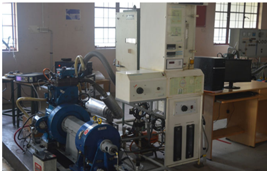
Fig. 1 Single-cylinder four-stroke CI engine with slaked calcium hydroxide solution setup
