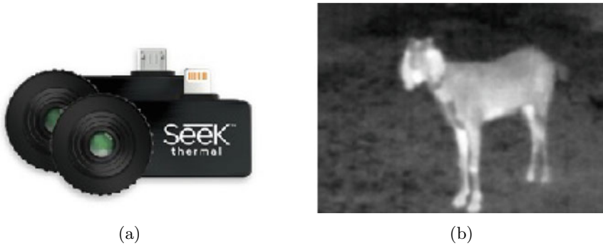
Fig. 1 IR imaging camera SeekThermal used for study. a IR sensor (compact); b grayscale image from IR sensor
