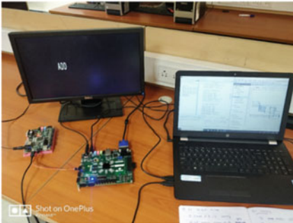
Fig. 11 Font display testing with font table stored in the SD card
