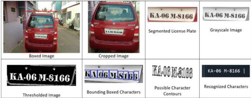
Fig. 18 Results of the proposed ALPR system with induced motion blur
