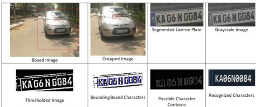
Fig. 17 Results of the proposed ALPR system under contrasting illumination conditions
