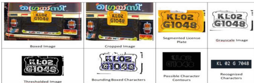
Fig. 20 Results of the proposed ALPR system with non-standard license plate text
