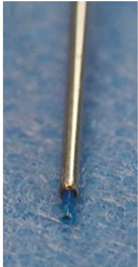
Fig. 21.13 (a) LISA LASER PRODUCTS Sphinx Jr. Holmium:YAG laser. (b) The laser fiber emerging from a metal protector
