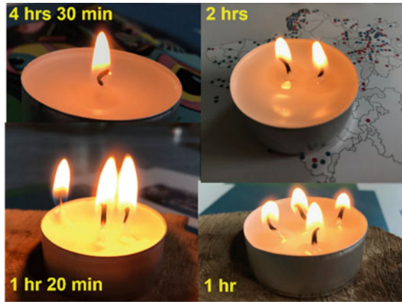
Fig. 3 Addition of wicks to increase the burning rate of a tea light candle
