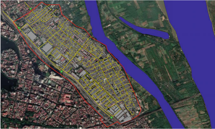
Fig. 3 Spatial data used to initialise the ESCAPE agent-based model on the Phuc Xa case study, including the ward boundary (red line), buildings (grey polygons), roads (yellow polylines), evacuation points (green circles), and the closest extends of the Red River (blue).
