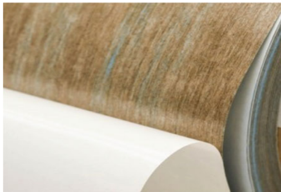
Fig. 4 Long flax fibers in thermoset reinforced sandwich panel ( https://www.castrocompositesshop.com/en/156-flax-epoxy )
