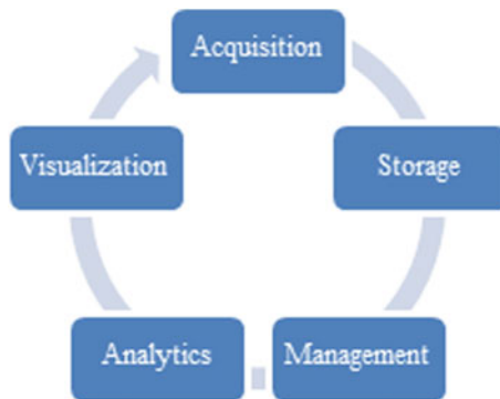
Fig. 1 Big data analysis process. The first step in the analysis process is data acquisition (data collected through different mediums and in different forms); the second step is to store the data; the third step is data management; and the fourth step is applying the analytic method to the data for extracting the meaningful information and at last data visualization is used for pictorial graphical representation
