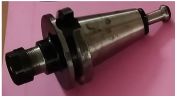
Fig. 3 View of burnishing tool attachment
