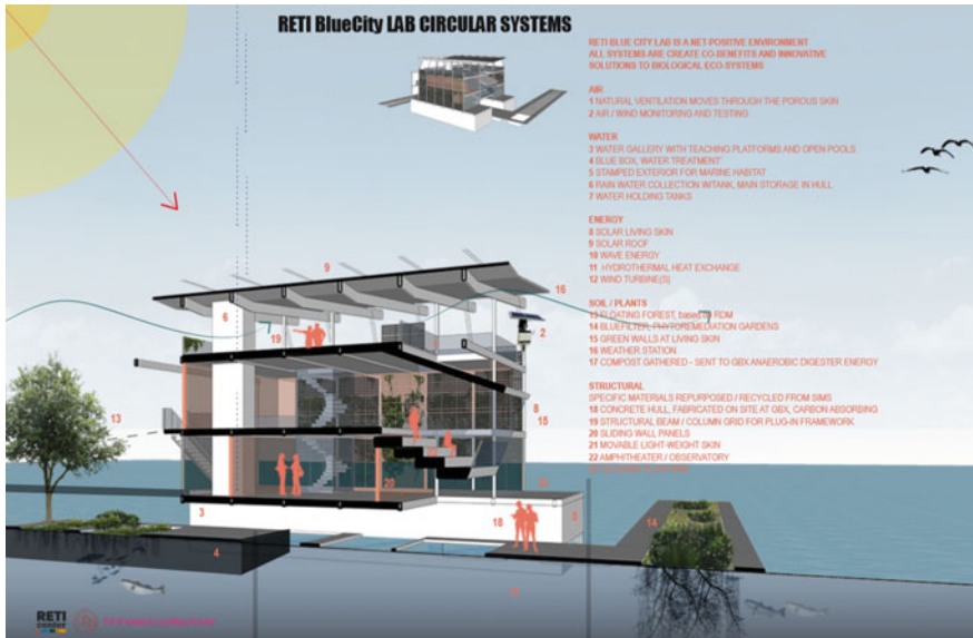
Fig. 11 Original conceptual programming/circular systems diagram for a larger iteration of BCL, thread collective + Oasis Design Lab
