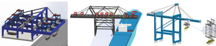
Fig. 4 Floating cranes design: rotate crane design ( left ), double-sided carrier crane ( center ) and feeder crane ( right )
