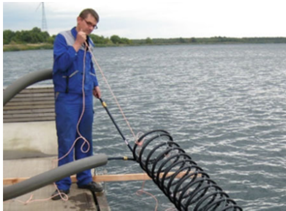
Fig. 2 Heat exchanger on the surface of a pontoon test samples with a simulation model
