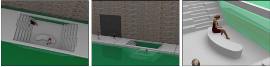
Fig. 2 Rendering of ecologically enhanced seawall elements and an underwater observatory
