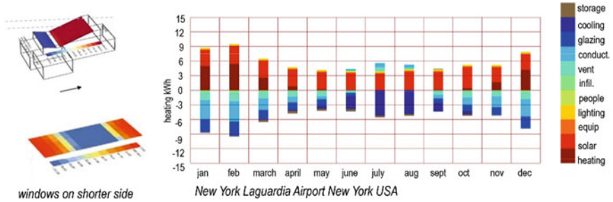
Fig. 9 Cooling/heating load with daylight autonomy calculations for orientation study, credit: Mrinalini Verma and Dorit Aviv, University of Pennsylvania (Studies performed in Ladybug/Honeybee Roudsari, M. “Ladybug + Honeybee.” Grasshopper. Np, nd Web 5 (2015), and Diva: Jakubiec, J. Alstan, and Christoph F. Reinhart. “DIVA 2.0: Integrating daylight and thermal simulations using Rhinoceros 3D, Daysim and EnergyPlus.” In Proceedings of building simulation, vol. 20, no. 11, pp. 2202–2209. 2011)
