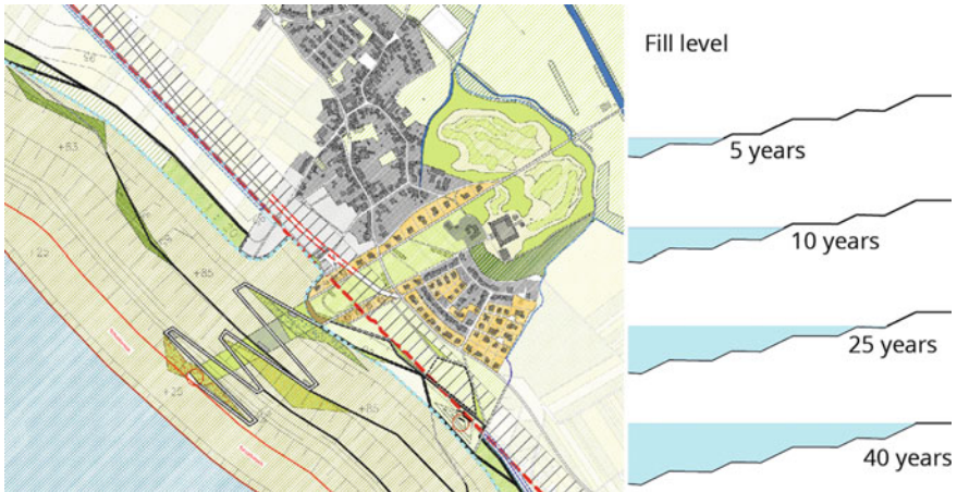
Fig. 5 Detail of the concept for village Schophoven and section with fill levels and berms after 5–40 years [11]
