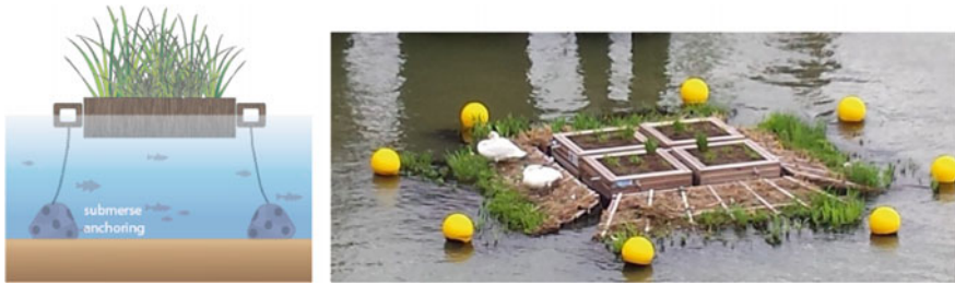
Fig. 9 Examples of floating green solutions (floating wetlands and gardens) that can potentially be combined with floating constructions for minimising undesired impacts of floating platforms and stimulating ecosystems and biodiversity
