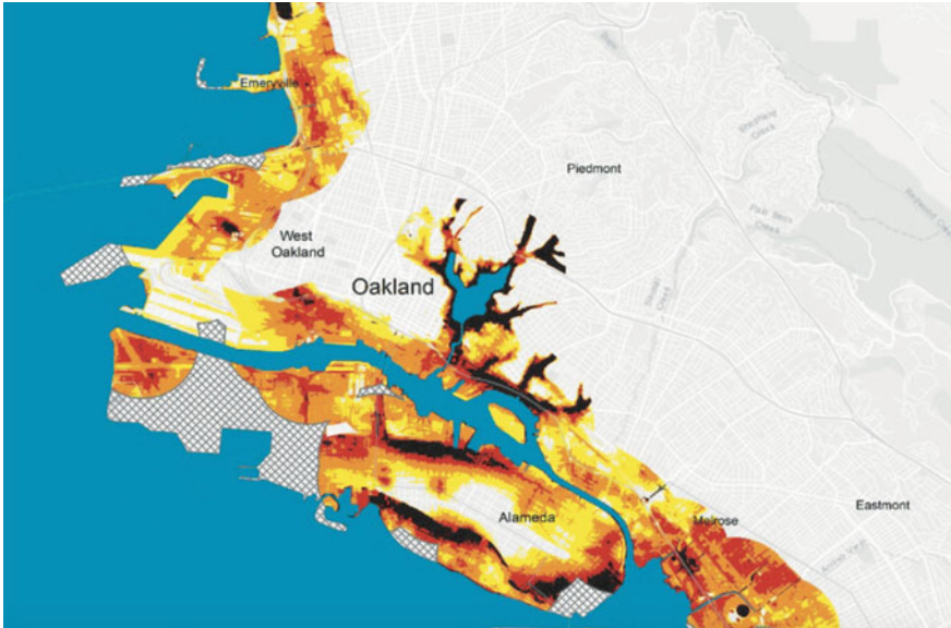
Fig. 3 Depth to groundwater under the cities of Alameda and Oakland, California, estimated by interpolation among well data points [8]. Black and red areas are likely to have groundwater within 1 m of the surface during wet conditions in 2020. Orange areas are likely to have groundwater within 2 m of the surface, and yellow are greater than 2 m in depth
