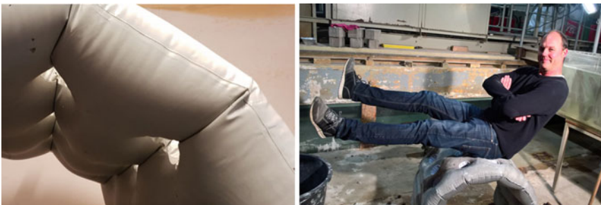
Fig. 5 Buoycrete demonstrator and 7-days UCS load test with 100 kg static load
