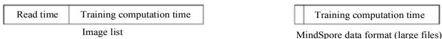
Fig. 14.3 Time consumption comparison between the conventional approach of reading an image list and the approach MindSpore uses
