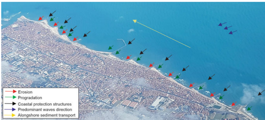
Fig. 7 Area photograph of coastal structures installed on the coastline of the Barra do Ceará and the Moura Brasil neighborhoods (west of Fortaleza. Aerial image courtesy of Everton Marinho)
