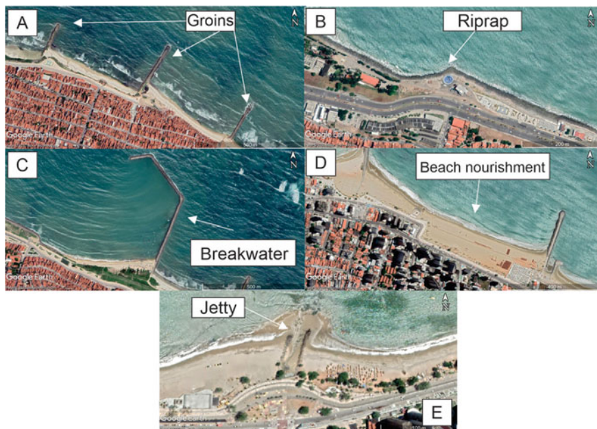
Fig. 4 Coastal structures on the coastline of the city of Fortaleza. a Groins in the Pirambu neighborhood; b Riprap installed in the Moura Brasil neighborhood; c Breakwater built in the Pirambu neighborhood; d Praia de Iracema Beach Nourishment; e Jetty in the Maceió stream, of the Mucuripe neighborhood
