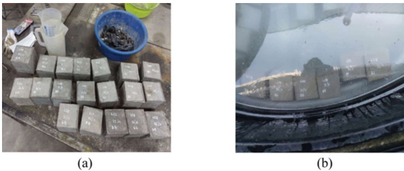
Fig. 1 Concrete specimen: a Cube specimen, b Curing process
