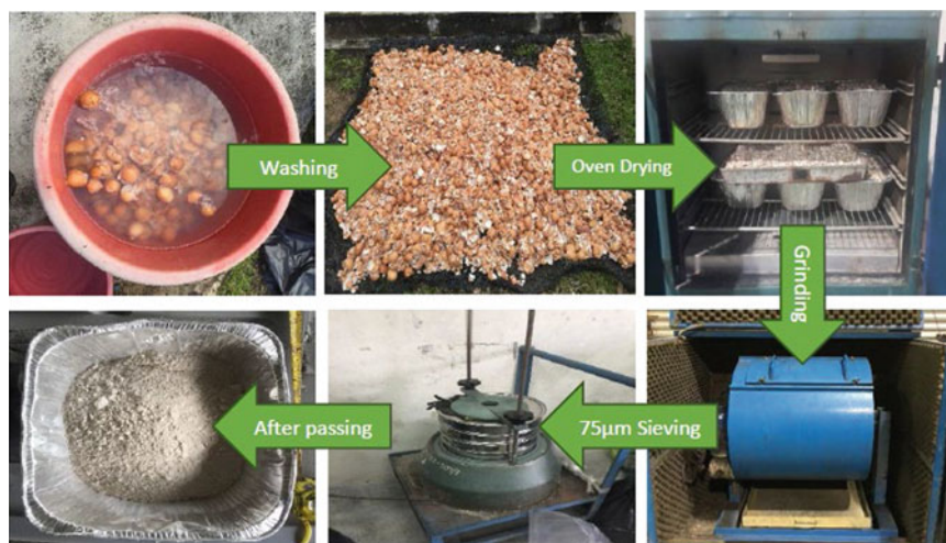
Fig. 3 Preparation of eggshell
