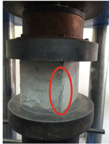
b) Pattern of crack on cube sample
