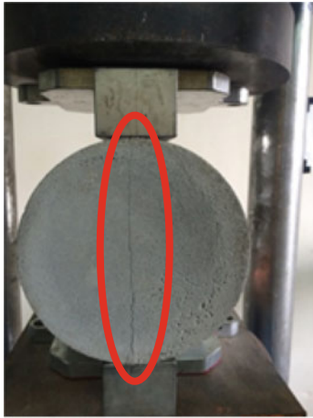
a) Pattern of crack on cylinder specimen
