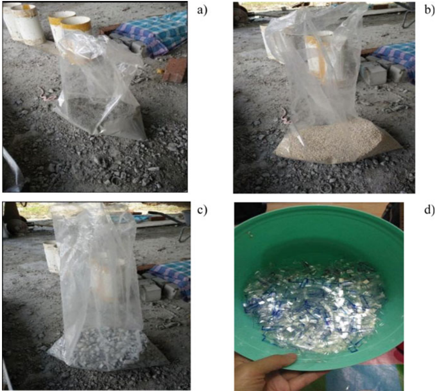
Fig. 1 Preparation of materials: a Cement, b Fine aggregate, c Coarse aggregate, d PET fibre
