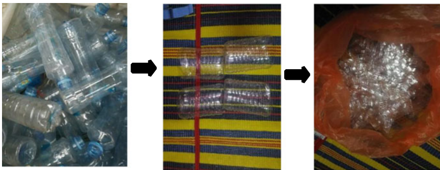
Fig. 2 The preparation of recycled PET fibres: a Collecting recycled PET plastic bottles, b Cleaning and drying recycled PET plastic bottles, c Cut recycled PET pieces into desired size and shape (25 mm long, 5 mm wide)
