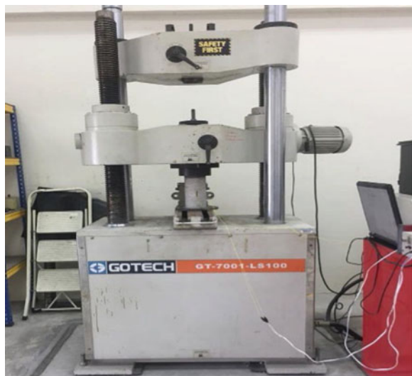
Fig. 4 Poisson's ratio and modulus of elasticity testing of cylinder
