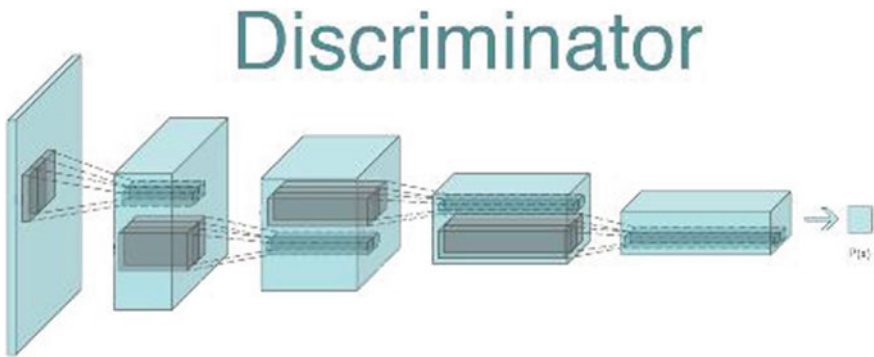
Fig. 2 Discriminator of a DCGAN with strided convolutional layers with the same dimensions
