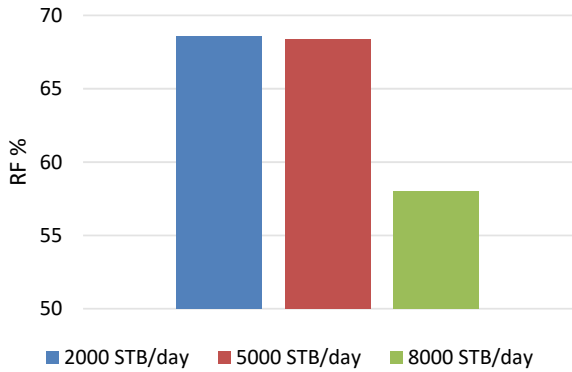
Fig. 5 Oil recovery factor at the end of simulation for the three different injection rates of CW
