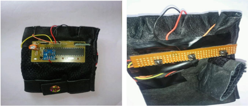
Fig. 1 Top and bottom view of hand data glove
