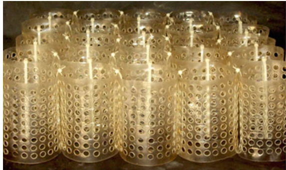
Fig. 1 Photograph of plastic bottle geocell mattress [7]
