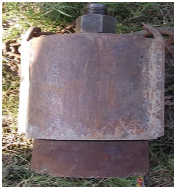
Fig. 1 Indigenous circular shape tamper
