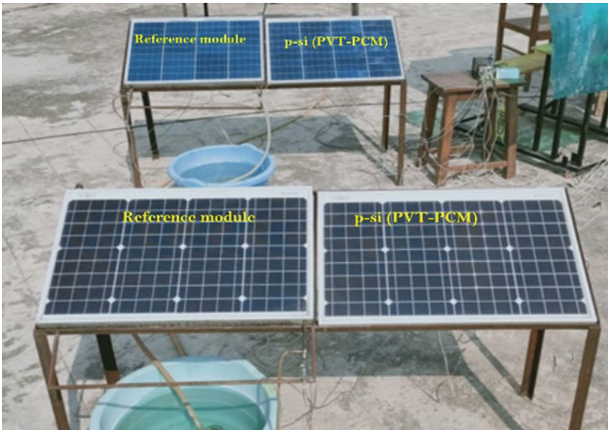
Fig. 1 Monocrystalline and polycrystalline-based PVT/PCM system with reference module
