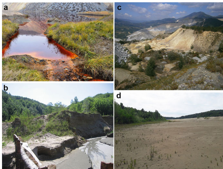
Fig. 9.1 Various types of generated mine wastes and possible environmental consequences: (a) sulfidic rock waste and generated acid mine drainage at Bor copper mine site; (b) Stolice antimony flotation tailing dam spill; (c) Veliki Krivelj copper mine waste rocks; (d) Flotation tailings of Rudnik polymetallic mine
