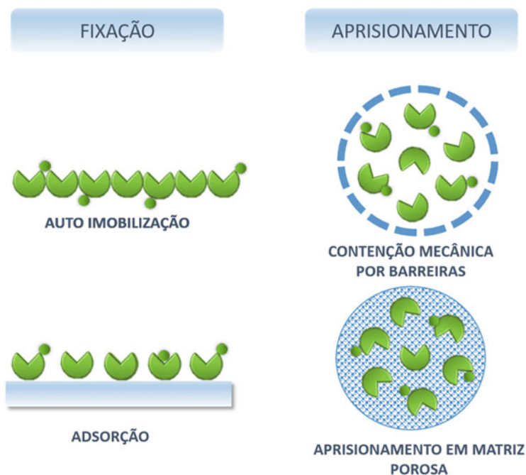
Fig. 7.4 Classification of immobilization methods
