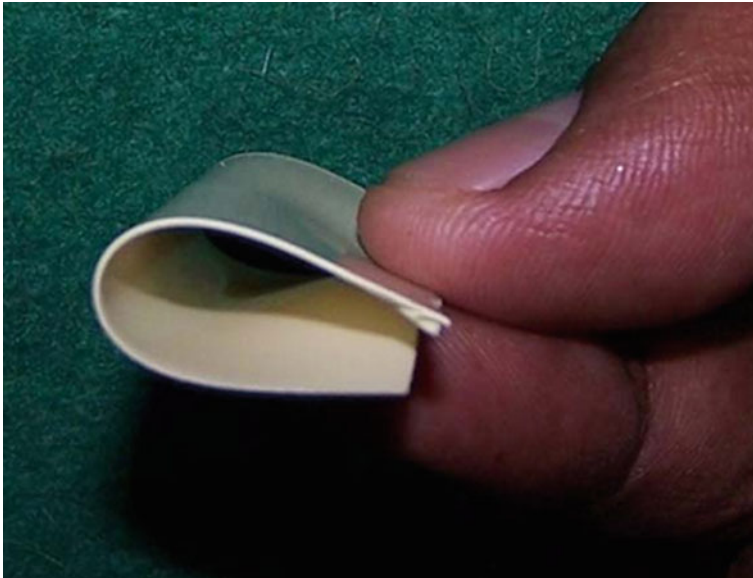
Fig. 1.16 Flexible radiation shield composite of PDMS-Bi 2 O 3 (30:70). “Reproduced with the permission of John Wiley and Sons” [55]
