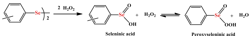
Scheme 13.55 Over oxidation of diaryl diselenides leading to seleninic and peroxy-seleninic acids formation
