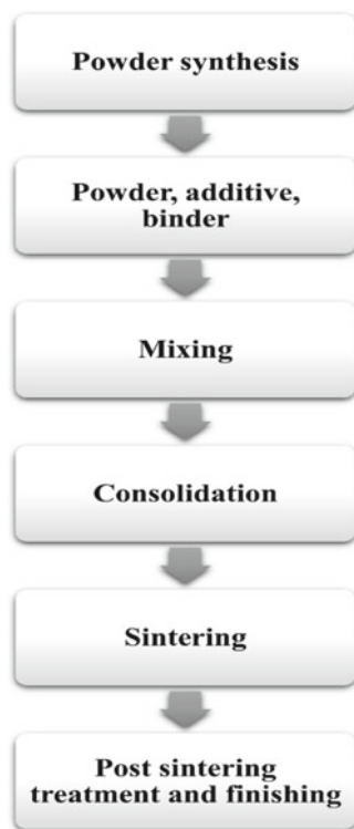
Fig. 18.12 General processing scheme for preparation of ceramic breeder
