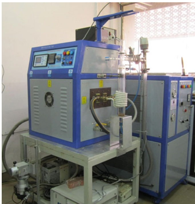
Fig. 15.4 Picture of a 12 kW induction furnace with accessories (in house fabricated)
