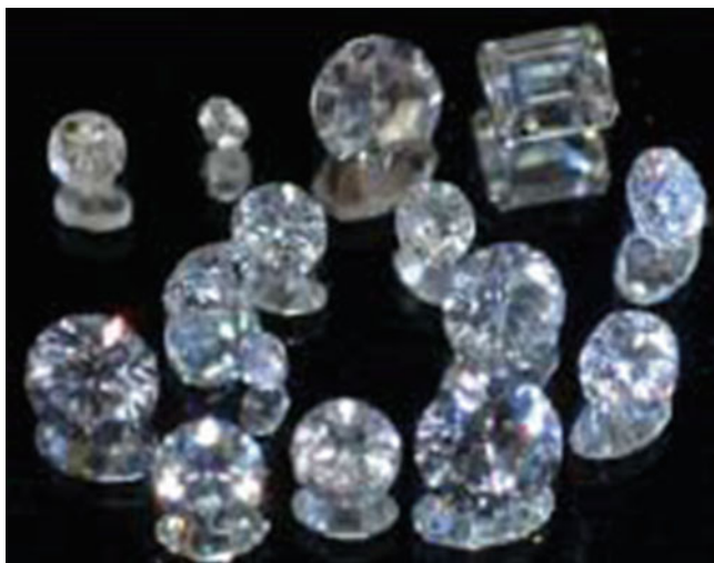
Fig. 10.7 Single-crystal diamond obtained by the 915 MHz microwave plasma CVD. The diamond crystal's weights were ranged from 0.2 to 1.15 carats (Reproduced with permissions [46]. Copyright 2014, American Chemical Society)
