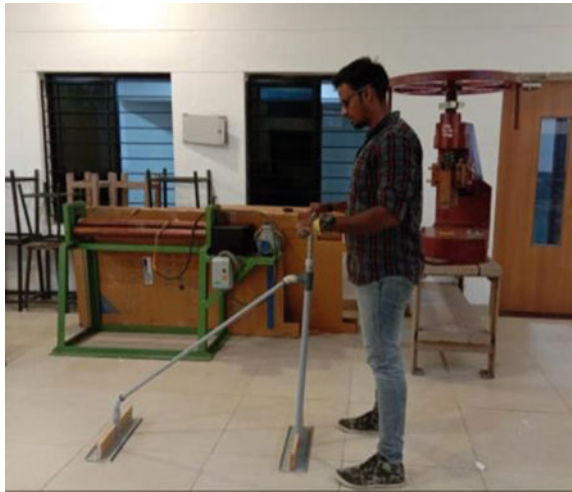
Fig. 16 Posture of a person testing an ergonomically designed model of a troweling tool
