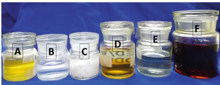
Fig. 9.1 The components used for biodiesel production ((a) WCO, (b) methanol, (c) Alkali) and finished products ((d) mixed product after the reaction, (e) biodiesel, and (f) glycerol)
