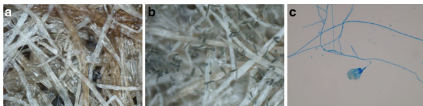
Fig. 1 Image of a panel sample before entering humidity and high temperature test (a). Image of a panel sample with fungi growth after 14 days exposure to humidity and temperature (b). Microscopy image of Aspergillus fumigatus (c)
