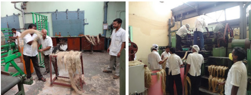
Fig. 5 Manual scutching and processing of flax waste fibre for spinning of high tenacity yarn [20, 21]
