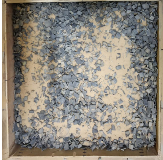
Fig. 6 Tire chip reinforced sand (Sample: TRS70A1B40)
