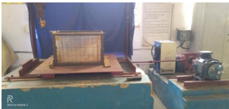
Fig. 1 Arrangement of the shake table instrument
