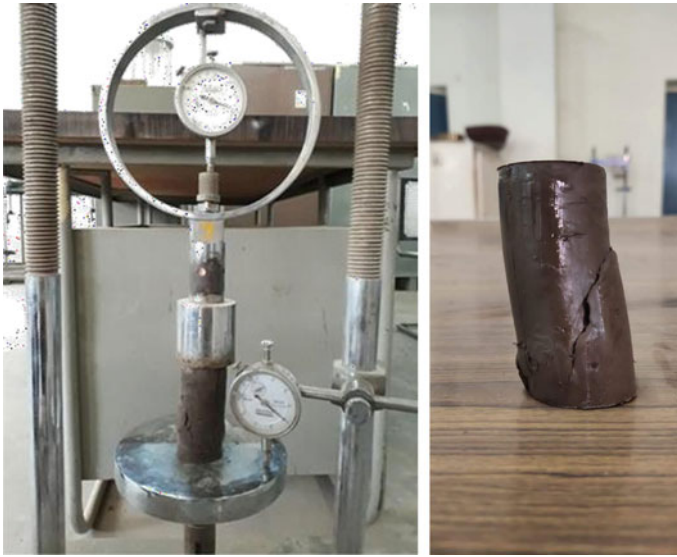
Fig. 8 UCS testing machine with sample
