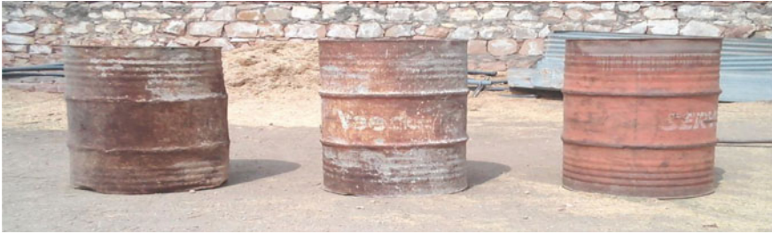
Fig. 2 Field arrangement showing empty diesel drums for in situ production of biochar
