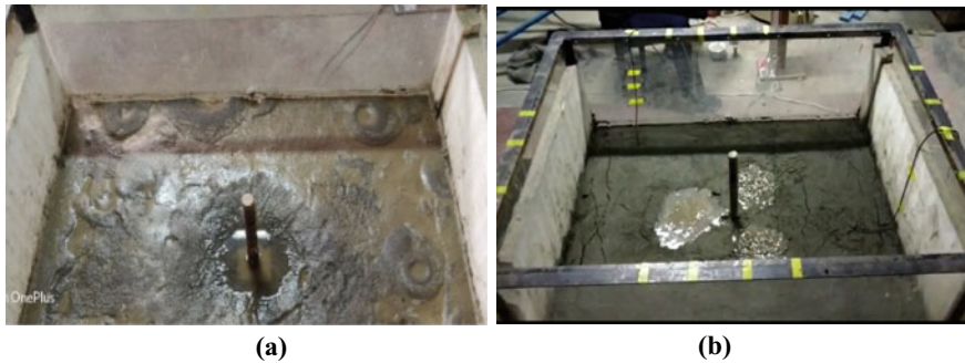
Fig. 5 a Sand boils depicting generation of EPWP in unreinforced bed. b Water seeping out initially from the gravel drains in SC reinforced bed
