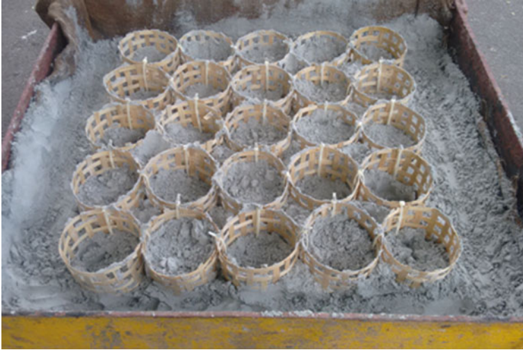
Fig. 6 Photograph of the preparation of bamboo cellular mattress reinforced fly ash bed
