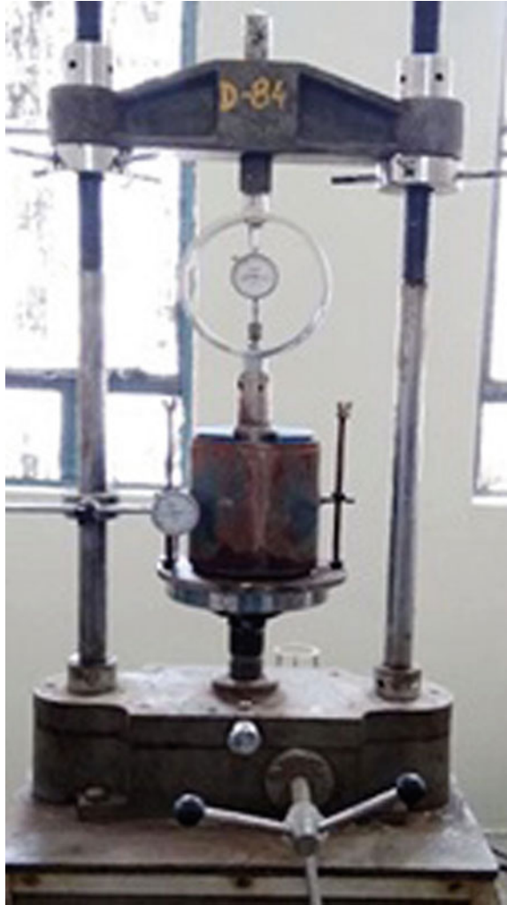
Fig. 10 California bearing ratio testing machine
