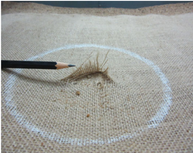
Fig. 4 Image of ruptured jute geotextile after the plate load test
