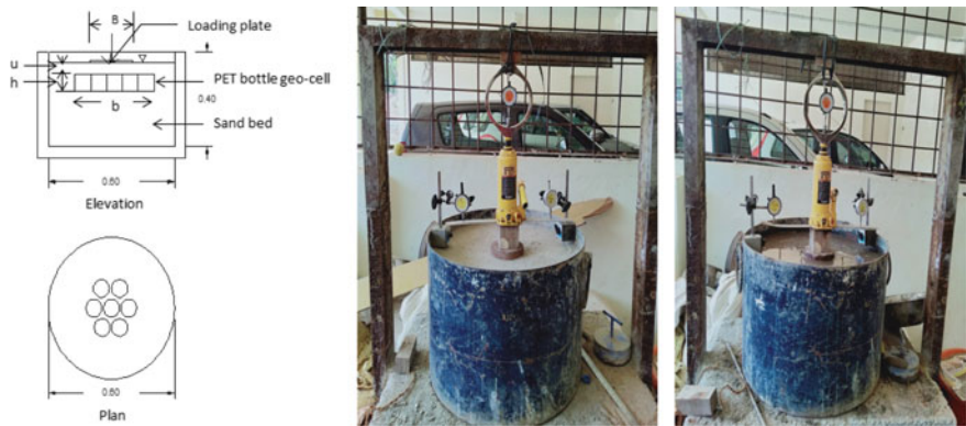
Fig. 1 Diagrammatic representation and image of the test setup under dry and submerged conditions
