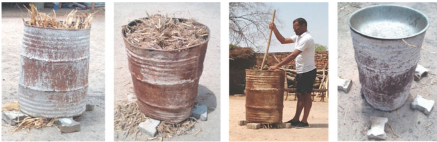
Fig. 3 Drums are filled with crop residues, compacted and covered with top lid after lit on fire at bottom and left for some time so that pyrolysis takes place
