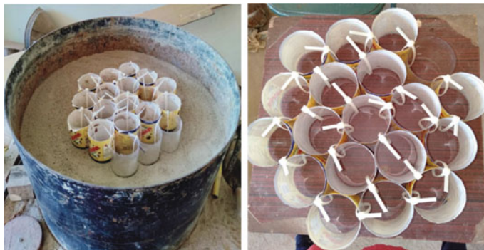
Fig. 2 Preparation of geocell-reinforced sand bed
