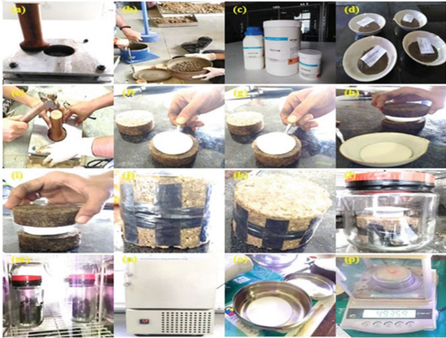
Fig. 2 Sequential sample preparation and filter paper test methodology
