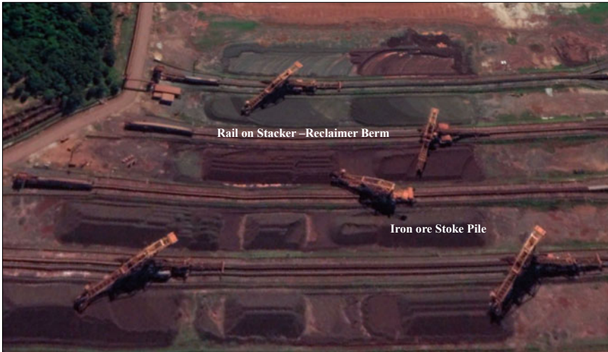
Fig. 1 Reference site picture with iron ore stockpile and stacker–reclaimer berm facility
