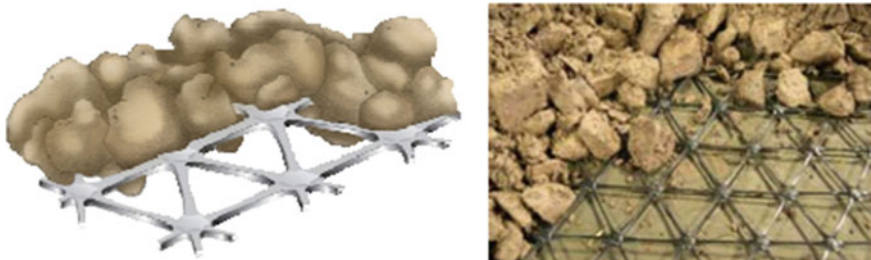
Fig. 1 Interlocking mechanism of stiff geogrid providing lateral confinement
