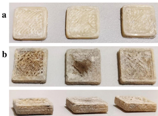
Fig. 13.7 3D structures of PHA (a) and 20TMP5E (b) after the degradation test: top and cross view (bottom)
