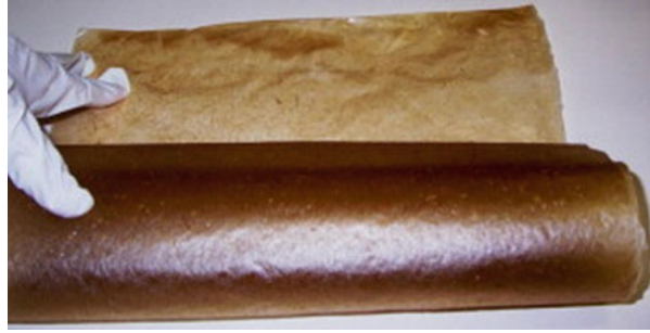
Fig. 4.5 Large dimension film prepared by tape-casting, containing 3 g starch/100 g of suspension, 0.20 g glycerol/g dry starch, and 0.30 g fibers/g dry starch. (Reprinted with permission from de Moraes et al. 2013)
