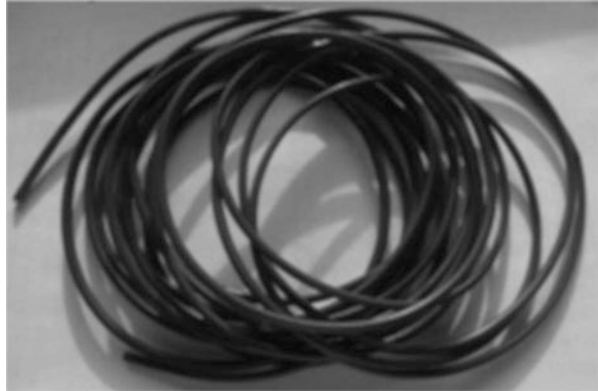
Fig. 4.1 Flexible tube obtained by extrusion of PLA bionanocomposite formulation. (Reprinted with permission from Rapa et al. 2019)
