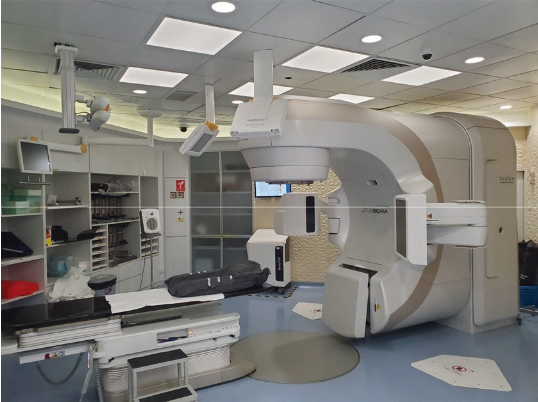
Fig. 1.1 A linear accelerator equipped with a cone-beam CT scanner and ExacTrac Adaptive Gating System housed in a thick-walled bunker
