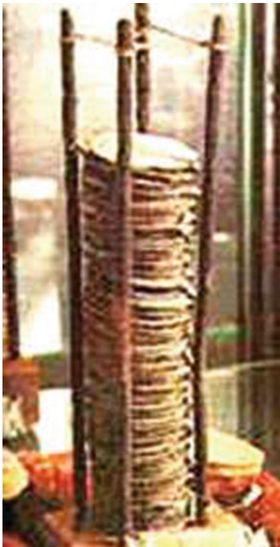
Fig. 14.2 A Voltaic Pile [reproduced with the permission of American Physical Society (Ref. [1]b, APS News, March 2006, vol. 15, No. 3)]
