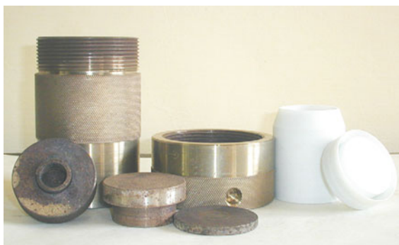
Fig. 5.2 Common variant of the autoclaves which is currently used in hydrothermal synthesis. [4] Reproduced with permission from Ref. Copyright 2007 Elsevier
