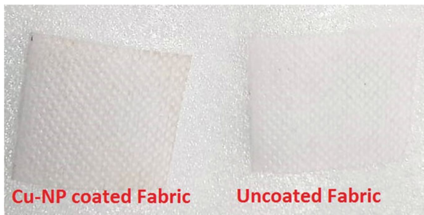
Fig. 20.8 Personal Protective Equipment (PPE) fabric coated with copper nanopowder produced by electrically exploded wire
