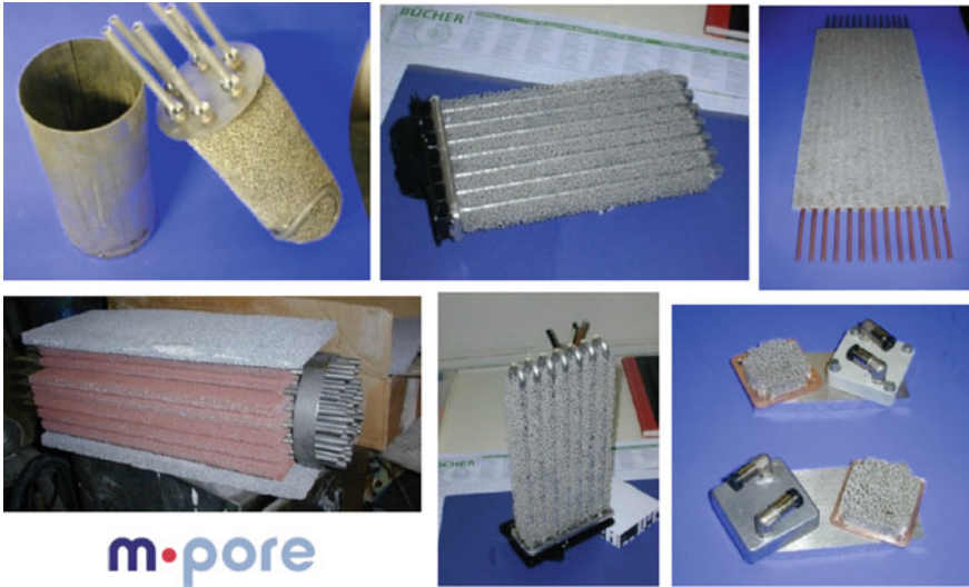
Fig. 9.10 Diverse types of heat exchangers based on Al- and Cu-foams manufactured by M. pore and Mayser GmbH, Reprinted with permission from Reference [309]. Copyright 2016 MDPI AG
