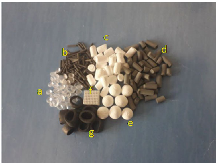
Fig. 17.2 Various shapes of catalysts for practical applications. a Granules b Extrudates c Pellets d Cylinders e Spheres f Monolith g Rings. Reproduced with permission from Ref. [37] Copyright 2018 MDPI
