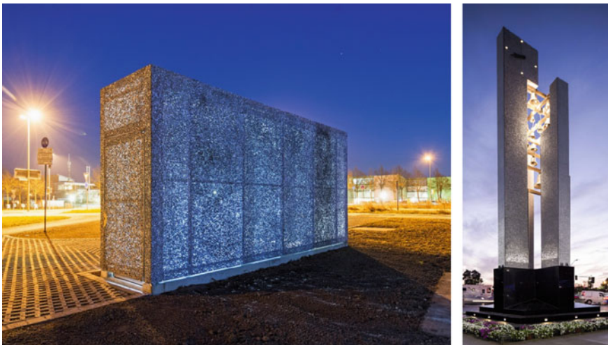
Fig. 9.11 Translucent entrance of a souterrain and bell tower monument made of Alusion foam, Reprinted with permission from Reference [309]. Copyright 2016 MDPI AG
