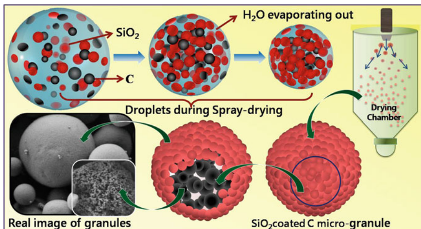
Fig. 11.22 Schematic representation of nano-composite core-shell micro-granules of carbon and silica. FESEM micrographs show silica-wrapped core-shell micro-granules and the carbon core after leaching. [42, 43] Reproduced with permission from Ref. (Reproduced from Ref. with permission from the Royal Society of Chemistry)
