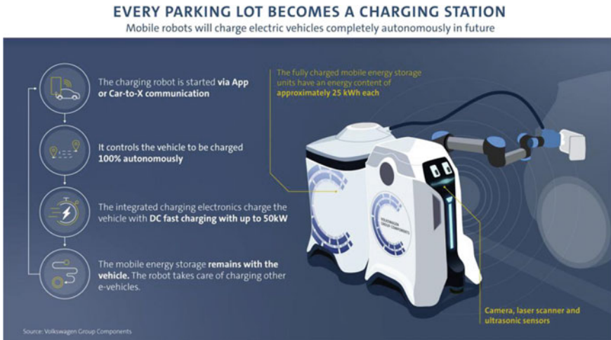
Fig. 1 Process of Volkswagen's autonomously charging mobile robots for EVs [9]
