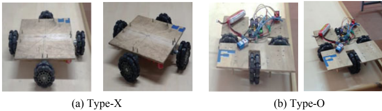
Fig. 8 Physical prototypes of the proposed 2-DOF translating mobile robots
