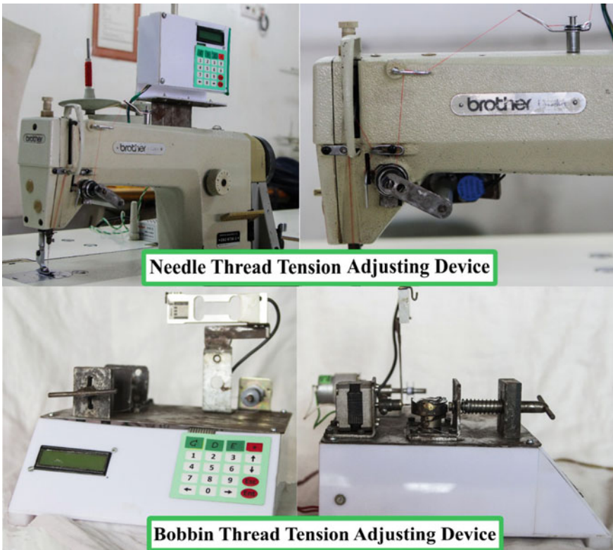
Fig. 5 Prototype of the thread tension adjustment device installed on an SLNS machine, at the garments construction laboratory, NIFT, Kolkata, India
