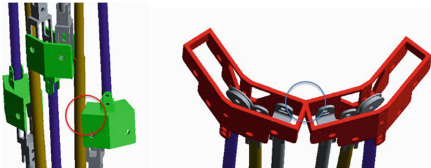
Fig. 6 CAD view of Interference of 3J joint body with diagonal member and 5J joints interfering with each other
