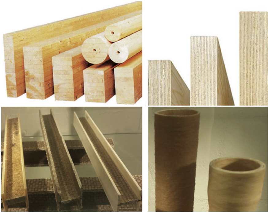
Fig. 3 Natural fiber composites for beams and columns in construction (Fan and Fu 2017)
