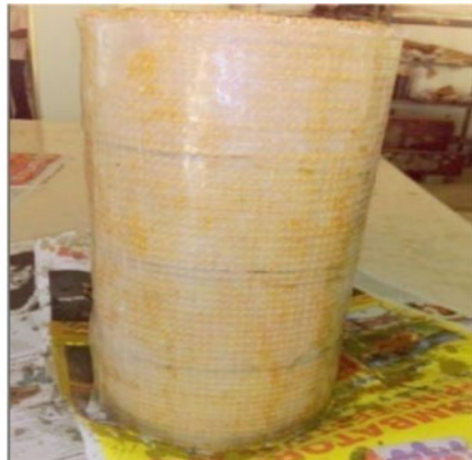
(b) cylinder wrapped with HSGFRP
