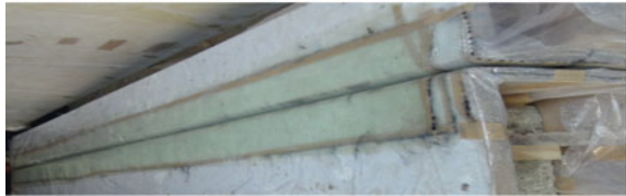
(c) Joining the two moulds together
