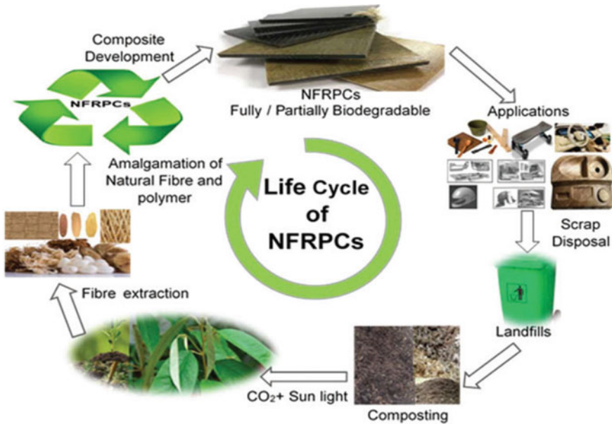
Fig. 2 Life cycle of Natural Fiber Reinforced Composites (NFRP) composites (Khan et al. 2018)
