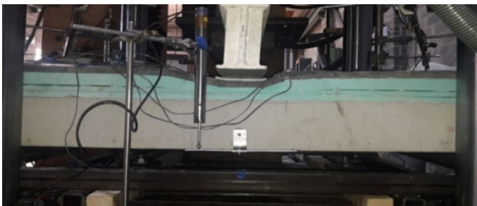
Fig. 21 The left and right wythe ends being restrained against uplift by the trussed CFRP connector in tension and insulation crushing under the load spreader due to local buckling of connector
