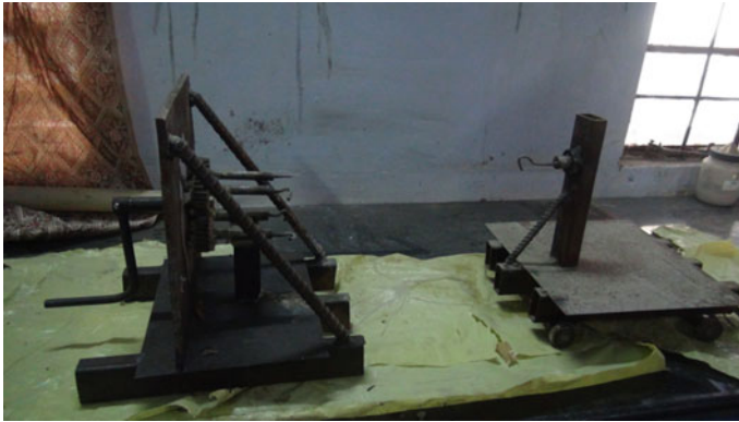
Fig. 1 Self-developed FRP bar manufacturing equipment
