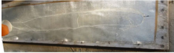
(a) Spreading of resin over fiber
