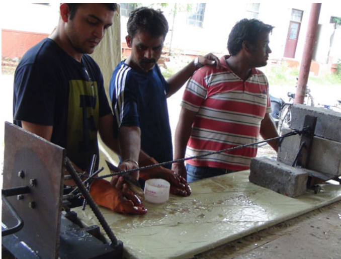
Fig. 2 Fabrication of CFRP bar
