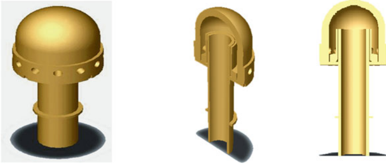
Fig. 44.3 Structure of combined blast cap
