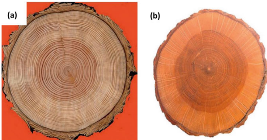
Fig. 2 The microstructure of wood (a) Coniferous Douglas Fir and (b) Deciduous English Oak (reused with permission, License number 4874720409441)
