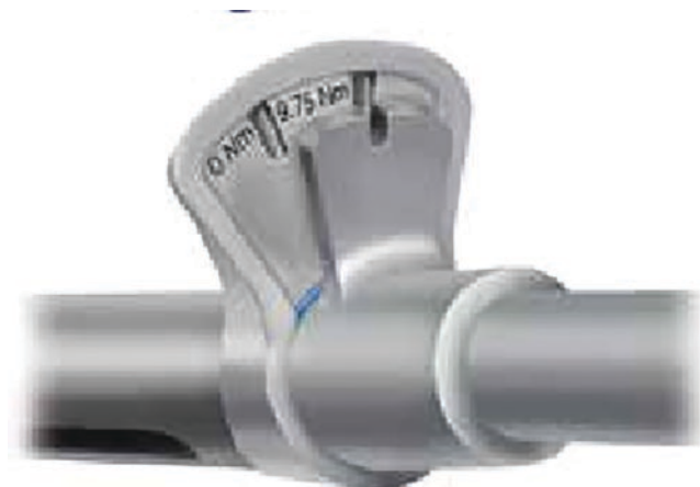
Fig. 9.30 The handle is turned until the slot reaches the line on the right side of the scale to ensure the Correct Torque limit has been achieved
