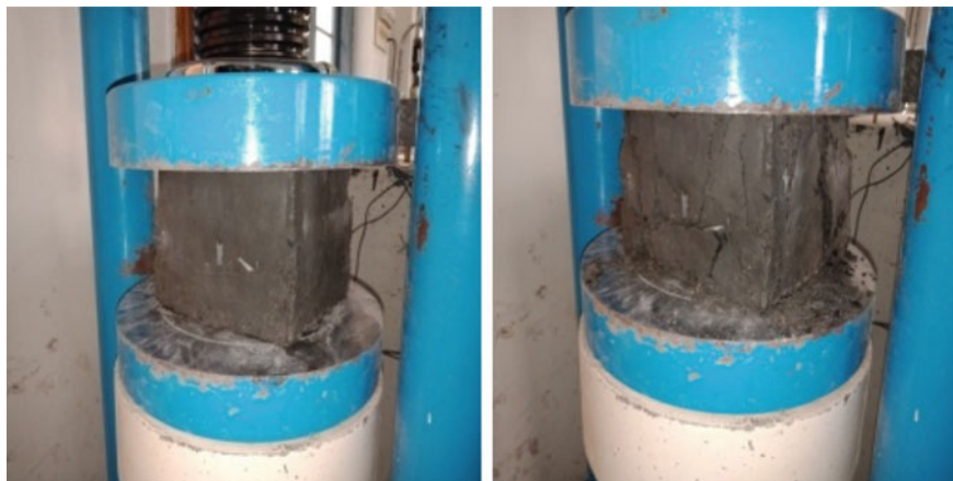
Fig. 5 Compressive test of fiber-reinforced concrete
