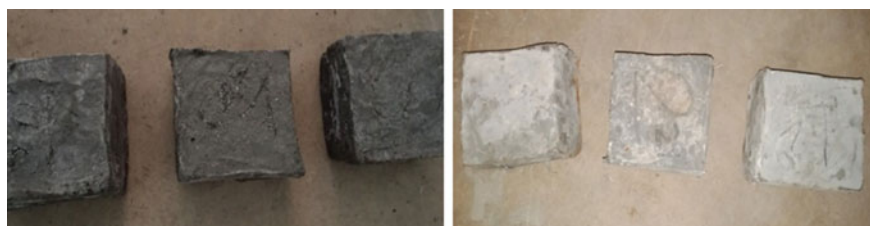
(a) PET-bottle reinforced concrete blocks
