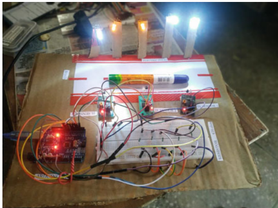
Fig. 11 When there are vehicles in front of all the streetlights at the same time
