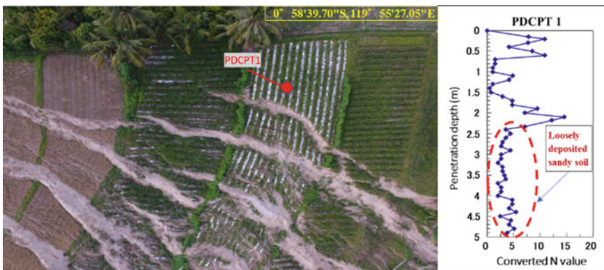
Fig. 12.13 PDCPT conducted near the crown of flow-slide and the test result (modified from Hazarika et al. 2020)
