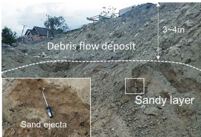
Fig. 12.25 Soil profile observed at the crown (Kiyota et al. 2020)
