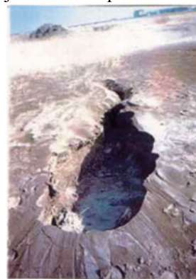
(b) Liquefaction and sand ejection in unimproved area
