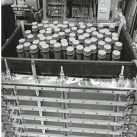
Fig. 3.49 1-G model test on effects of rigid columns on mitigative effect of liquefaction (Bahmanpour et al. 2019)
