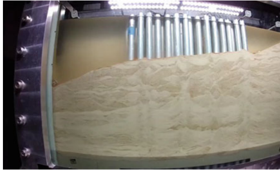
Fig. 3.51 Mitigation of lateral flow of liquefied slope by installed vertical columns (photograph was taken by the author) (Towhata et al. 2015)
