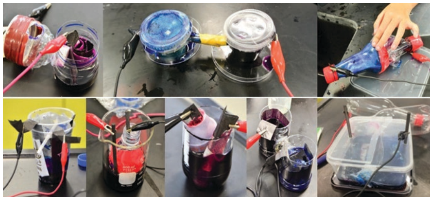
Fig. 11.6 Examples of student-built microbial fuel cells
